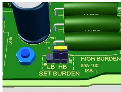
Figure 2: Link for setting operating burden
